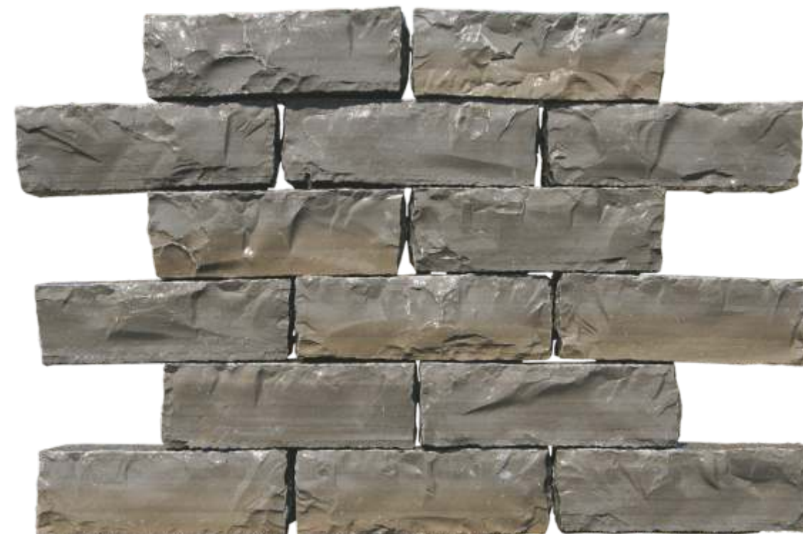
Wall Bricks: Top Surface Natural, Bottom Surface Calibrated, Sides Hand cut. (40 X 20 X 8cm)
